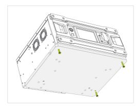
5. Mount the adapter plate ZEL-MKS-024 at the bottom of the Zeliox Compact with 3 bolts.
