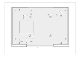
3. Place adapter ZEL-MKS-020 inside drawer and check the spacing around the plate, this should be equal.
