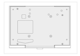
Place adapter ZEL-MKS-020 inside drawer and check the spacing around the plate, this should be equal.
