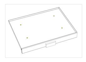
4. Drill 4 holes size 7mm at the marked positions.
