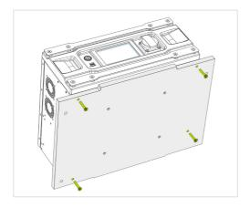
5. Mount the adapter plate ZEL-MKS-020 at the bottom of the Zeliox Compact.
