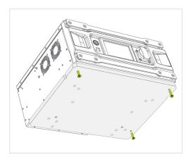
6. Mount the adapter plate ZEL-MKS-024 at the bottom of the Zeliox Compact with 3 bolts.
