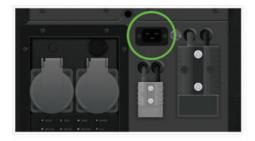
2) switch off Zeliox by clicking the Power Switch
