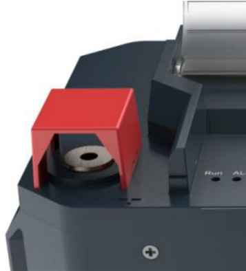
Figure 2-7 - Remove the protective cover of the lithium battery
